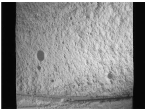
Fig. 3. Micrograph of fracture surface showing large air bubbles, potential sites of secondary cracking (sample thickness is 20 mm).
